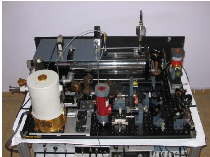
Figure 1: View of the infrared tunable diode laser spectrometer used for the quantification of formaldehyde.
