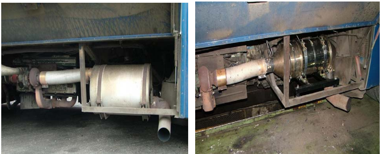
Figure 2: Rába D10UTSLL160 diesel engine with the original silencer (left) and with Baumot BA1012 particle filter (right) in a bus of Ikarus 280.40 type
